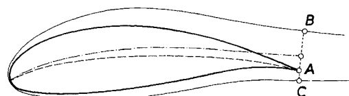
Fig. 1 Equivalent airfoil contour, generated by adding the boundary-layer thickness to the original shape.
